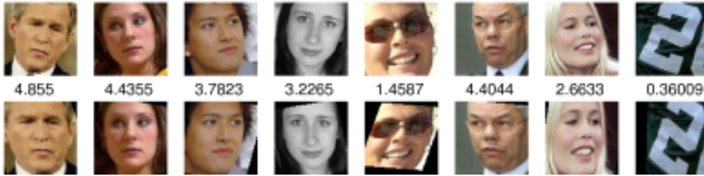
Figure 3: The face detector can detect faces in a range of orientations, as the top row shows. Before clustering the face images we rectify them to a canonical pose bottom row . The faces are rectified using a set of SVM's trained to detect feature points on each face. Using gradient descent on SVM outputs, the best affine transformation is found to map detected feature points to canonical locations. Final rectification scores for each of these faces are shown center (where larger scores indicate better performance). This means that incorrect detections, like the rightmost image can be discarded because of their poor rectification scores.
