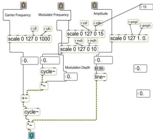
Figure 9: Frequency Modulation
