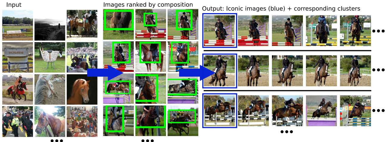
Figure 2. The flow of our system: Left: Large pools of images from the web are collected for a specified object category (a random set returned for the query “horse” are shown here). Notice that many of these images do not show the object category or provide unsatisfactory depictions. Center: In a single linear pass images are ranked according to a category independent composition model that predicts whether they contain a large clearly delineated object of any category, and outputs an estimated location of that salient object (green boxes). Only the most highly ranked images are retained for more expensive pairwise local feature comparisons. Right: Local features calculated on the proposed object regions are used to eliminate objects not distinctive to the category, and to cluster images by similarity of object appearance. Resulting iconic images are shown outlined in blue followed by images with similar object appearance to the right.
